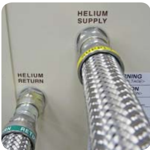
F-70 Compressor flex hose connections
