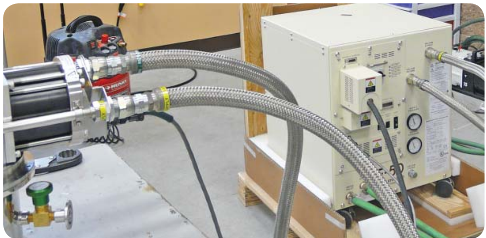
Cryocooler Coldhead connected to compressor
